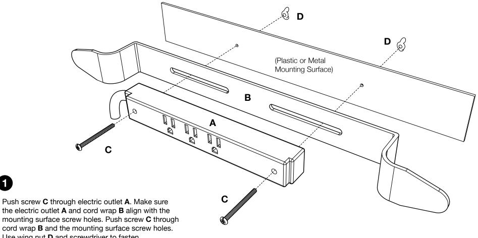
Use wing nut  $\ensuremath{\textbf{D}}$  and screwdriver to fasten.
