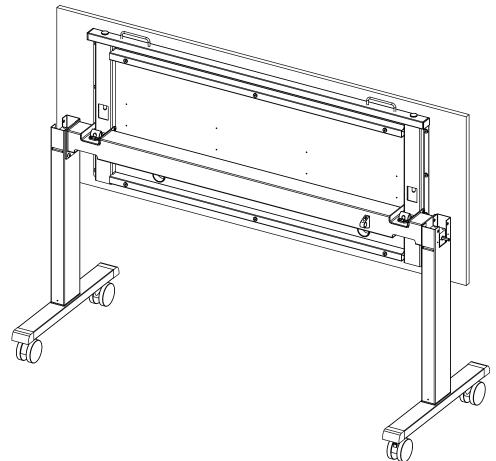
Step 6: Gather screws (J) and the M5 hex wrench. Finish attaching legs (B & C) to the top frame (A) with 2 screws (J) per side, using the M5 hex wrench.
