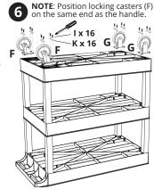
Flip unit upright after casters are securely installed.
