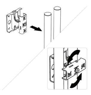
Adjust bracket to desired height and lock into place with provided wrench.
