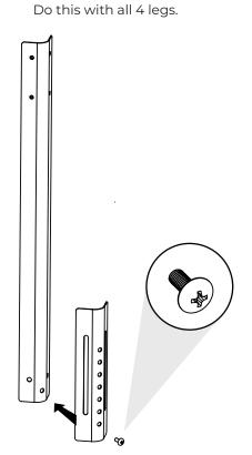
Insert all 4 legs into the upper cabinet. Secure using 4 Philips head screws (M6x16mm) per leg.
